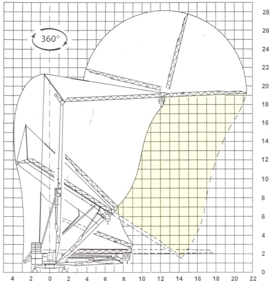
**Assembling:** Positioning and leveling on 360° - Assembling in few minutes in narrow places - Automated oleodynamic assembling with aerial opening of the jib - Remote-controlled independent movements of assembling - Safety valves on the whole system - Microswitch oil level in the gearbox
