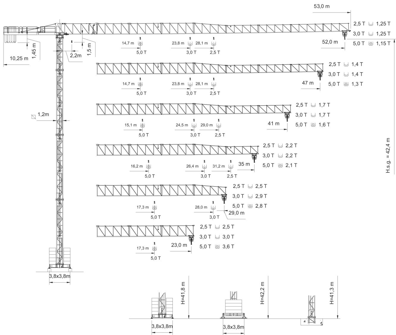
curve di carico cargo curves load diagrams courbes de charges
